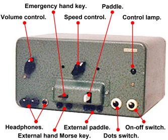
Layout of front panel with explanation of the control functions.
